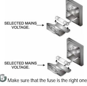
Battery charger ALTAIR WBPC-200 set up to 230 V.
